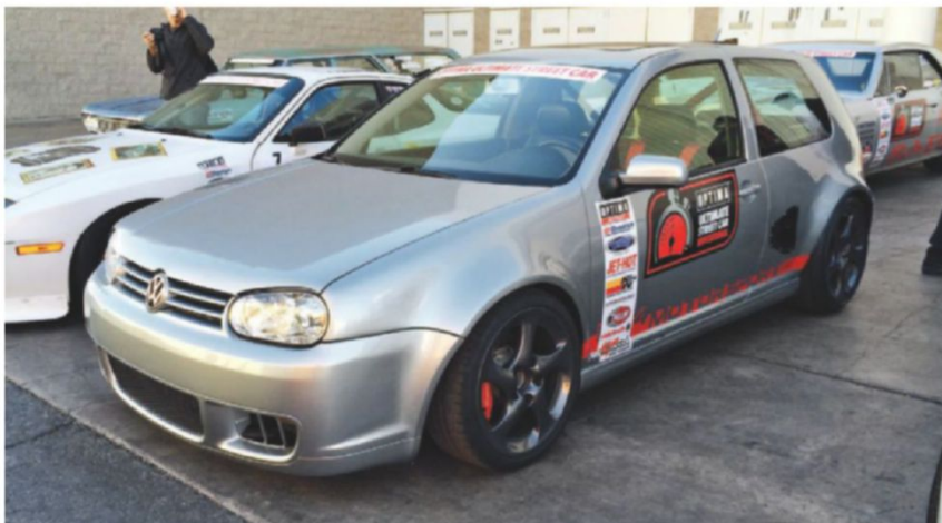
The GTI RS from Q34 Motorsport may be the wildest Golf on the planet. An Audi turbocharged V-6 sits in the middle of the car, feeding power to the rear wheels.
