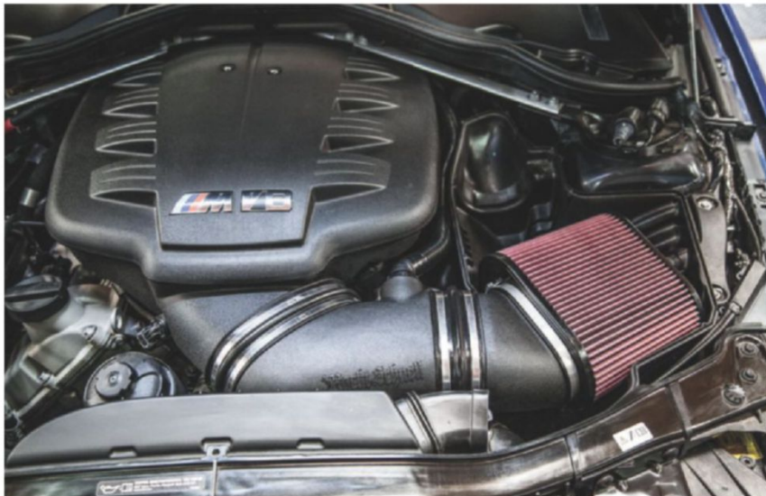
Connect the charge pipe to the intake manifold plenum, followed by the air-inlet adapter, air filter, and airbox lower. Make sure and secure all of the clamps before installing the airbox lid. Here's a peek at just how gargantuan the new intake system is.
