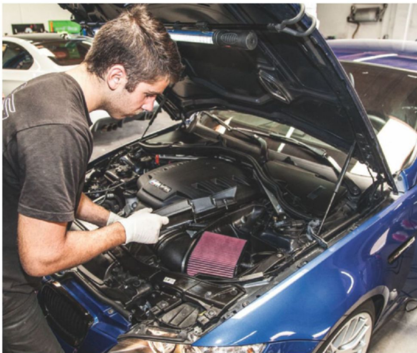
Next, you'll want to install the airbox lid and secure all of the factory bolts.
